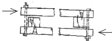
the planks so that when the bolts are removed and planks are gently struck with wooden mallets in opposite directions as shown by the arrows these end blocks come away with them. If the planks used are not of adequate section they will be forced out in the centre when ramming the concrete but this can be counteracted by giving them lateral support.
